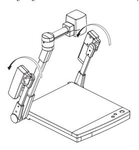
7. Lower the right lighting arm and rotate the camera head to its original position.
